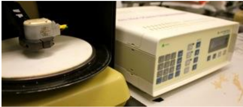
Figure 4.2: Four-Point Probe used for Resistivity Measurements of SiC [6]
