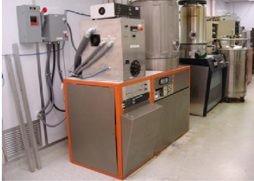
Figure 2.10: Resistive Heating Evaporator Located in the NCSU Cleanroom [5]
