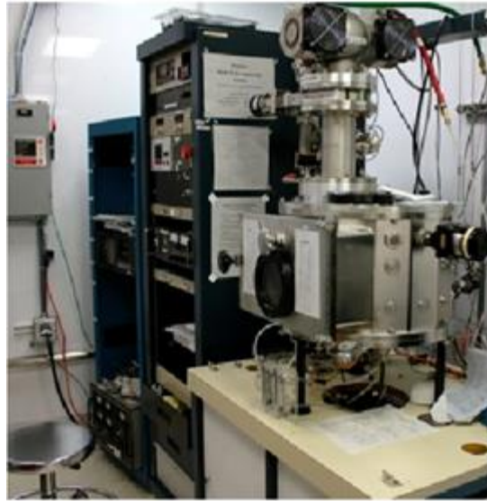
Figure 2.11: DC Sputtering used to Deposit Gold Contacts
